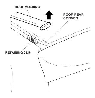
If the front or rear retaining clips remained on the roof molding, remove them from the roof molding, and reinstall them in their original positions on the vehicle. Remove the remaining clips and set them aside; they will not be reused.
