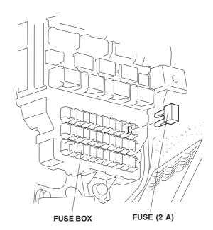
60. Attach the fuse label to the No. 33 slot on the fuse box cover.
