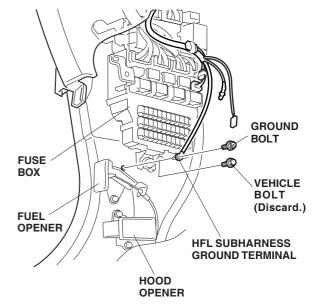
17. Disconnect the vehicle harness 1-pin connector and connect it to the HFL subharness 1-pin connector.
