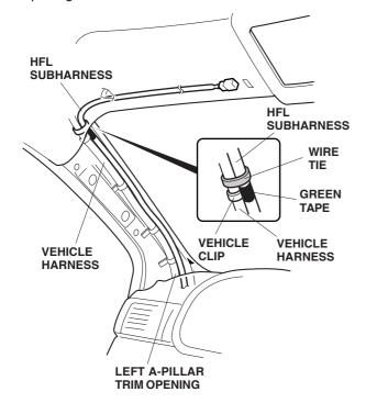
15. Route the HFL subharness and secure the harness to the vehicle harness with a wire tie above the vehicle clip as shown.
