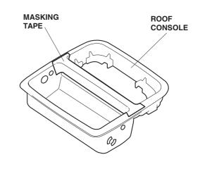
30. Attach template A with masking tape to the roof console at the indicated position.
