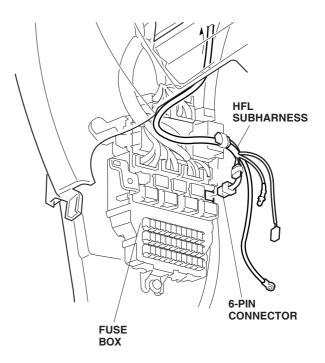
NOTE: If another accessory is already plugged into the 6-pin connector, remove the dummy connector from the 6-pin connector taped to the HFL subharness. Plug the 6-pin connector from the other accessory harness into the 6-pin connector from the HFL subharness you just unplugged and plug the HFL subharness into the fuse box.
