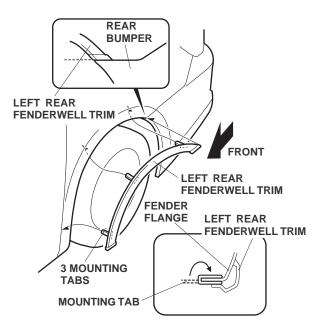
9. Using a rubber mallet, install the inner protector over the fender flange and fenderwell trim.
