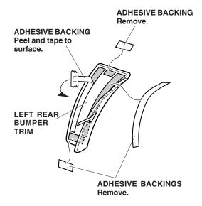
11. Using an alcohol swab, thoroughly clean the area where the left rear bumper trim will install. Align the edge of the left rear bumper trim with the edge of the left rear fender as shown. While applying light pressure against the left rear bumper trim, carefully remove the taped adhesive backing.
