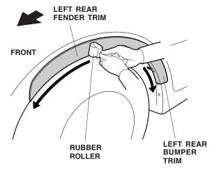
13. Hold the left rear fender trim upward and bend the mounting tabs around the left rear fender. Use needle-nose pliers wrapped in a shop towel to bend the mounting tab around the fender flange. Repeat for the left rear bumper trim.
