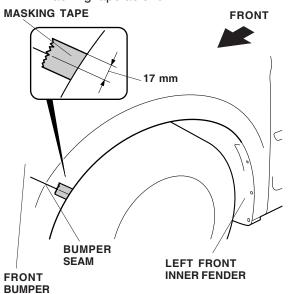
2. Peel back the adhesive backing from the upper part of the left front fender trim and tape it to the surface. Remove the remaining adhesive backings from the left front fender trim.
