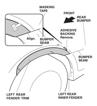
Peel back the adhesive backing from the upper part of the left rear bumper trim and tape it to the surface. Remove the remaining adhesive backings from the left rear bumper trim.
