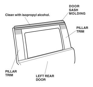
On the back of the left rear door visor, peel back 1 to 1 1/2 inches (26–38 mm) of the adhesive backings, and tape them to the front surface of the left rear door visor with a masking tape.
