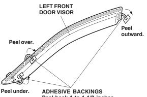
Peel back 1 to 1 1/2 inches (26–38 mm) from the adhesive tapes and tape them to the front of the left front door visor. 4. Position the left front door visor on the left front door. There should be approximately 5 mm between the end of the left front door visor and the end of the pillar trim.
