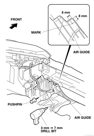
21. While wearing an eye protection, drill the pierced mark to 7 mm. First drill with a 3 mm drill bit, and finish with a 7 mm drill.
