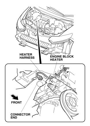
11. Route the heater harness up, and secure the two wire ties with clip (points A and B) to the bracket.
