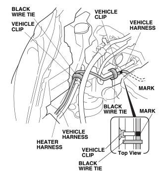
Route the heater harness as shown and secure the two wire ties with clips (points C and D) to the vehicle frame.
