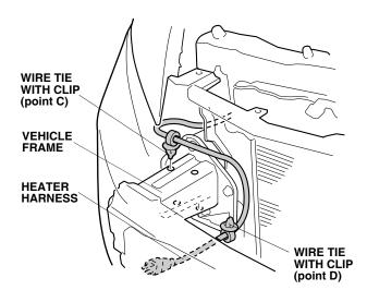
16. Bundle the excess of the heater harness. Using three black wire ties, secure the harness to the vehicle harness.
