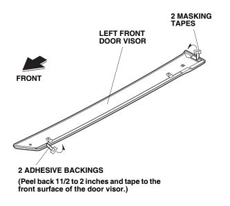
4. Using isopropyl alcohol, clean the door sash on the driver's door where the left front door visor will attach. Allow the alcohol to dry.
