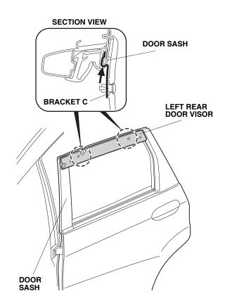
29. Insert bracket D between the rear pillar trim and the door sash, and insert the bracket E between the rear door center trim and the door sash. Install the left rear door visor on the door sash using the two clips. Verify the shape and the identification mark stamped on each bracket.
