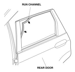
13. Remove the rear door run channel in the area shown.
