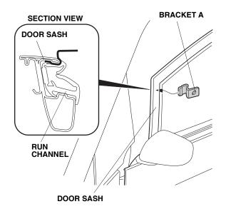
6. Temporarily install the left front door visor on the door sash using the two brackets C you installed on the left front door visor.
