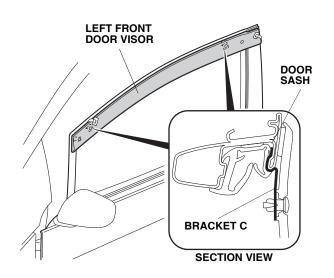
7. Push the left front door visor forward and up, and check that it aligns with the contour of the door sash. There should be no clearance between the brackets and the door sash.
