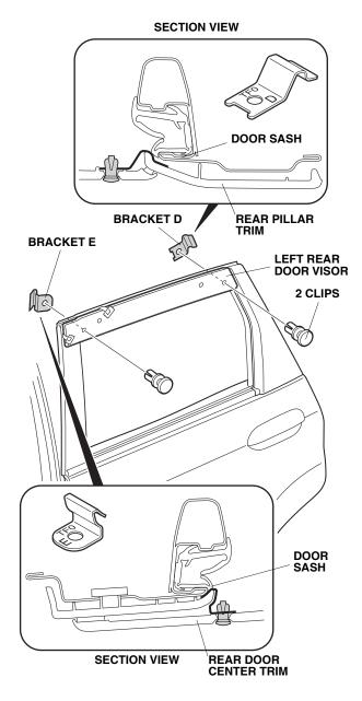
30. While holding the door visor up firmly and aligned in the center, remove the adhesive backings. Use your finger to push up on each bracket so there is no gap between the brackets and the door sash.
