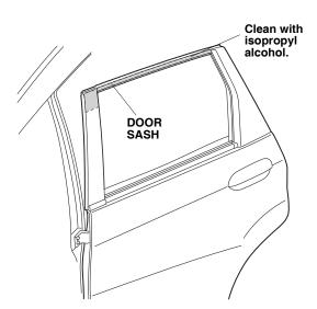
27. Temporarily install the left rear door visor on the door sash using the two brackets C you installed on the left rear door visor.
