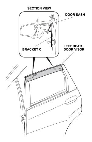
28. Push the left rear door visor upward, and check that it aligns with the contour of the door. There should be no clearance between the bracket and the door sash.
