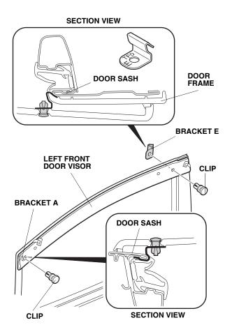
9. Adjust bracket A up or down until the hole in the bracket lines up with the hole in the door visor, and install a clip.
