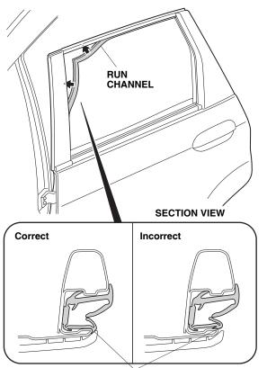
Check that the run channel is installed properly.
