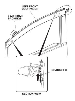
11. Using a soft towel, press and hold the door visor against the door sash for 30 seconds.
