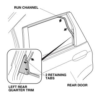
19. Carefully release the rear door run channel in the area shown. The run channel can tear easily at the corner area.
