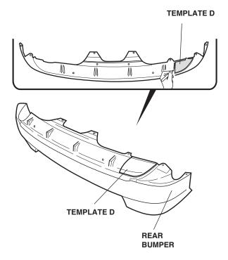
9. Using an airsaw, cut the rear bumper along the line. Use a file to remove any burrs from the edge.
