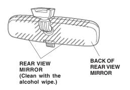
Remove and discard all of the adhesive backings from inside the mirror cover, and attach the mirror cover to the rear view mirror. Press and hold the mirror cover firmly against the mirror for 30 seconds.
