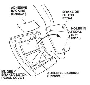
9. Remove the adhesive backing from one Mugen brake/clutch pedal cover. Align the top of the pedal cover over the brake or clutch pedal, and press the pedal cover into the pedal in the position shown above.
