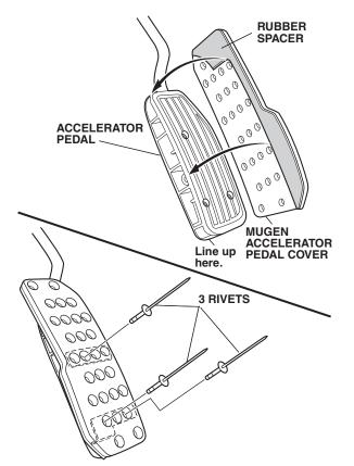
6. Place one spacer on each rivet. Using the rivet tool, compress each rivet while holding the spacer tight against the pedal. Remove the spacers.
