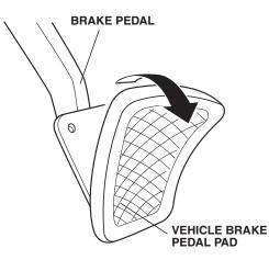
8. Using isopropyl alcohol on a shop towel, clean the brake/clutch pedal. Allow the alcohol to dry.
