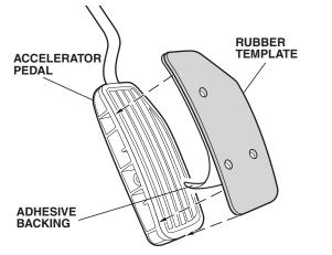
2. Using a pushpin, pierce the accelerator pedal at the center of each hole in the rubber template. Remove the rubber template.
