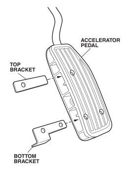
5. Place the Mugen accelerator pedal cover over the accelerator pedal with the top edge and the side edge of the rubber spacer tight against the pedal. Insert the three rivets through the pedal, the brackets, and the pedal cover at the holes shown.
