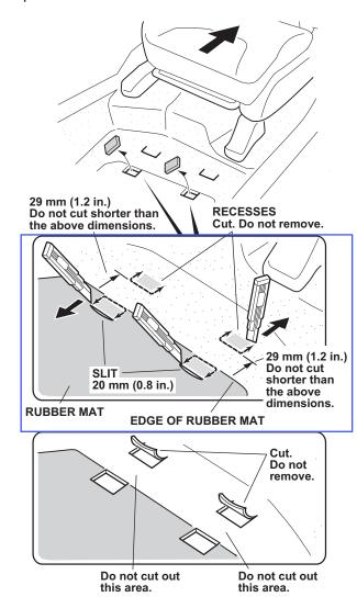
3. Locate the two recesses in the carpet. Using a utility knife, slit the carpet at the front of the recess in the direction shown. Be careful not to cut out the piece between the recess and the rubber mat, otherwise the entire floor carpet must be replaced.
