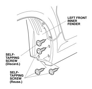
4. Place the left front splash guard on the left inner fender as shown.
