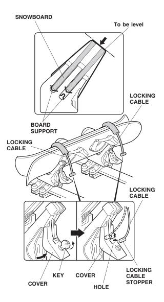
Check that the plate is inserted into the slit securely. Check that the locking cable is inserted in the groove securely.
