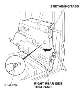
15. Remove and discard the cover from the right rear side trim panel. Slide the accessory socket protector into the vacant hole and align the tab on the protector with the cutout in the panel.
