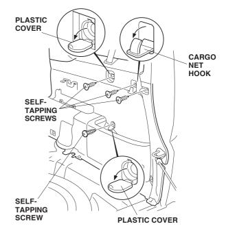
13. Remove the right rear bulkhead cover from the right rear side trim panel (eight retaining tabs).
