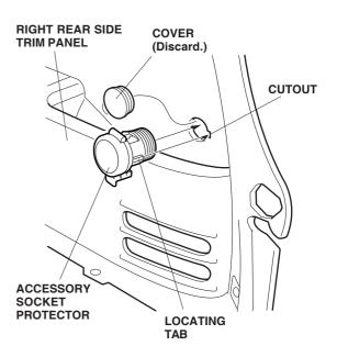
16. Open the lid, then slide the accessory socket into the accessory socket protector and align the tab with the cutout in the protector.
