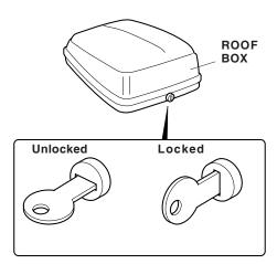
**Locking**: Press down on the lid. You should hear an audible click. Be sure the lid is latched by attempting to lift the lid. Turn the key clockwise to lock the roof box. Remove the key while not in use. Be sure the straps are not outside of the roof box.
