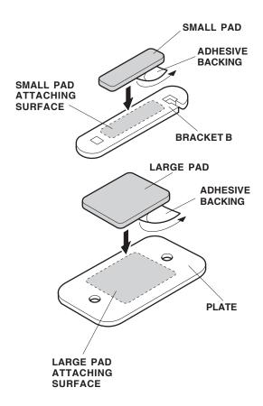
Using isopropyl alcohol on a shop towel, clean the four plates where the large pads will attach.
