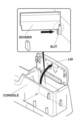
2. Turn the divider on the slit of the console and align the other end of the divider with another slit.
