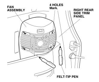
4. Using a felt-tip pen, mark the right rear side trim panel through the four holes in the fan.
