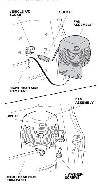
9. With the ignition on, use the fan switch to test the operation of the fan.
