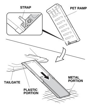
Place the plastic portion of the loading ramp on the tailgate, and the extended metal portion on stable level ground. 3. When finished using the loading ramp, slide the extended end into the top. Attach the strap to secure the two halves together.
