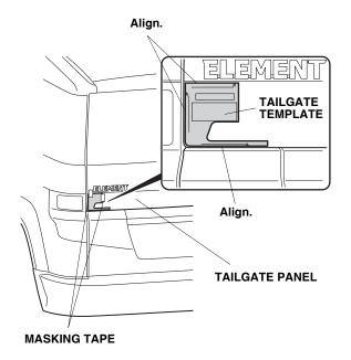
2. Get the tailgate emblem. Peel back  $1\frac{1}{2}$  - 2 inches of adhesive backing from the emblem, and tape it to the front of the emblem with a strip of masking tape.
