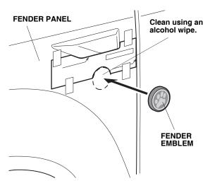
10. Place the fender emblem on the fender panel and align top edge of the emblem with the lower edge of the fender template.
