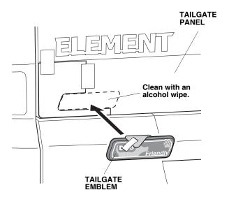
4. Place the tailgate emblem on the tailgate panel, and fit the emblem into the template as shown.
