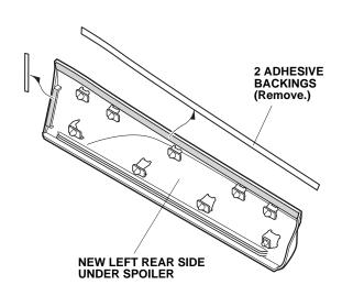
10. Hold the new left rear side under spoiler up, and install the trim seal to the door panel first. Fit the nine clips into the holes in the body, then push on the side under spoiler until the clips snap into place.
