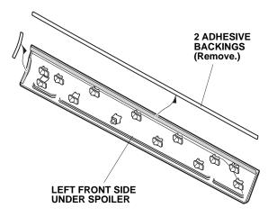
13. Hold the new left front side under spoiler up, and install the trim seal to the door panel. Fit the 13 clips into the holes in the body, then push on the left front side under spoiler until the clips snap into place.
