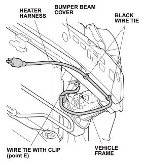
22. Using two black wire ties, secure the heater harness to the bumper beam cover.
