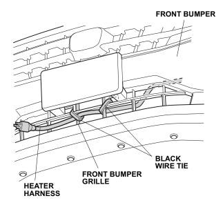
24. Attach the protective cap to the front bumper grille, and plug the heater harness connector into the protective cap.
