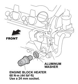
16. Plug the connector end of the heater harness into the engine block heater.
