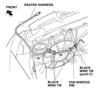
19. Using three black wire ties, secure the heater harness to the fan shroud ribs.
