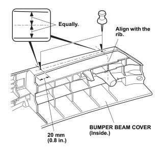
9. While wearing eye protection, drill the bumper beam at the pierced marks cover as shown. Wrap duct tape around a 5 mm drill bit 10 mm (0.4 in.) from the tip.
