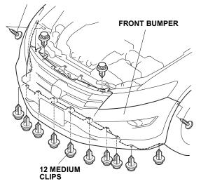
With the help of an assistant, remove the front bumper (unplug the two vehicle connectors).
