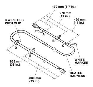
13. Using a white marker, measure and mark the heater harness at the measurements shown.
