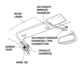
23. Secure the day/night mirror harness to the vehicle harness with one wire tie at the green tape.
