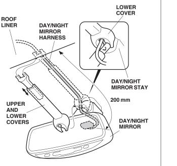
26. Slide the upper cover up under the roof liner.
