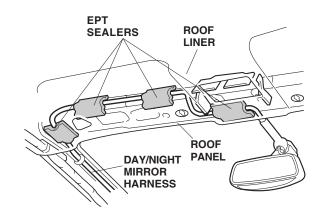
28. Secure the day/night mirror harness to the vehicle harness with three wire ties in the areas shown.
