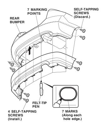
10. While applying pressure to the rear under spoiler, use a felt-tip pen to mark the rear bumper along each hole edge in the bracket on the rear under spoiler.
