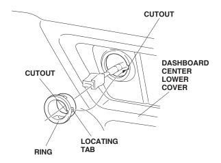
Align the locating tab on the socket with the cutout in the ring, and slide the socket into the ring.
