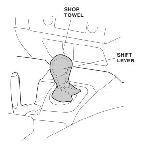
Shift to 2nd gear. Remove the lid from the dashboard center lower cover (four retaining tabs).
