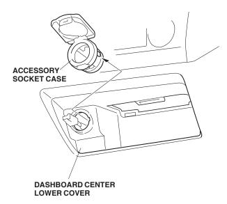
8. Connect the vehicle 2-pin connector to the new socket.
