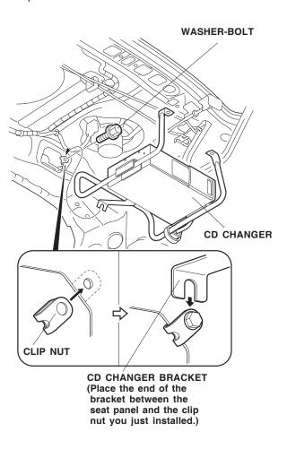
35. Loosely install the washer-bolt to the rear seat panel first. Place the end of the CD changer bracket between the seat panel and the clip nut you just installed.
