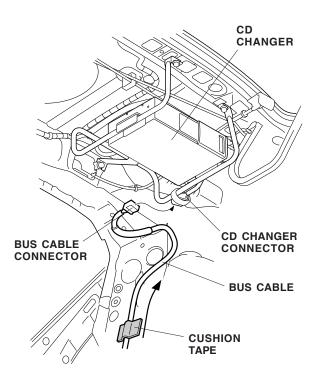
38. Fold the excess bus cable, and secure it to the holes in the rear seat panel with the two wire ties with clip.
