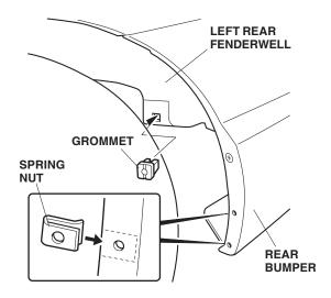
7. Position the left rear splash guard on the left rear fenderwell and rear bumper, then install the two 5 x 25 mm self-tapping screws and one 5 x 20 mm self-tapping screw. Tighten the three self-tapping screws in the order shown cut off any excessive under coat material with a utility knife.
