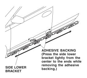
When the workshop room temperature is below  $60^{\circ}F$  ( $15^{\circ}C$ ), warm up the entire side lower bracket to  $60^{\circ}F$  ( $15^{\circ}C$ ) or above before attaching it to the vehicle body.
