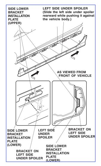
20. Check that all six brackets of the left side under spoiler are set in the side lower bracket installation plates.
