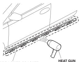
SIDE LOWER BRACKET (Warm up the side lower bracket when the workshop room temperature is below 60°F [15°C].)
