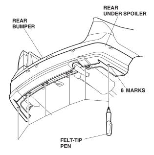
NOTE: If a gap is visible between the rear bumper and under spoiler, remove the under spoiler and confirm the locations of the marks with a tape measure. If necessary, create new marks in the proper locations.
