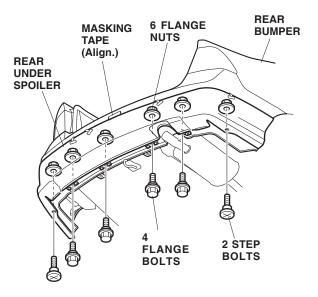
13. Check that the top edge of the rear under spoiler aligns with the lower edge of the masking tape you attached in step 1, and remove the masking tape.
