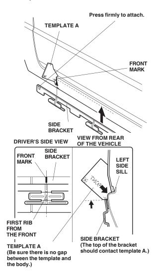
12. While wearing gloves, press the front portion of the side bracket (where you removed the adhesive backing) firmly against the vehicle body so that the adhesive will adhere.
