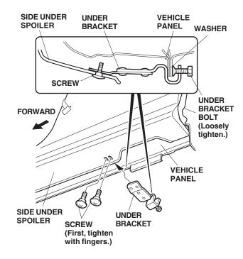
27. Position the under bracket on the side under spoiler and loosely install the two screws. Loosely tighten the under bracket bolts.
