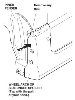
25. Loosely install the front self-tapping screws in the holes on the wheel arch of the side under spoiler.
