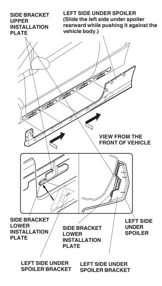
21. Check that all six brackets on the left side under spoiler are set in the side bracket installation plates. Visually check that there is no excessive gap between the left under spoiler and the vehicle. If you can see a gap, repeat step 20. 22. Attach the under bracket to the side under spoiler and mark the under coat.
