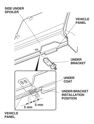
23. Using a utility knife, cut the under coat at the marked location, and file off the under coat from both sides of the vehicle panel.
