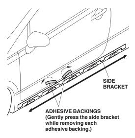
16. While wearing gloves, attach the side bracket to the vehicle body by pressing firmly along the double-sided adhesive tape with the palms of your hands.
