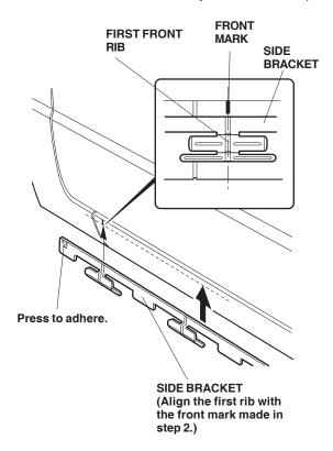
8. While wearing gloves, temporarily attach the side bracket to the vehicle body by pressing on the front of the side bracket where you removed the adhesive backing.
