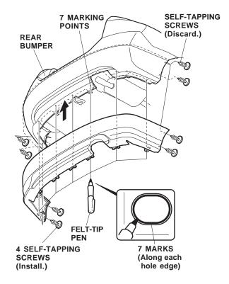
While holding pressure on the rear under spoiler, use a felt-tip pen to mark the rear bumper along each hole edge in the bracket on the rear under spoiler. NOTE: If a gap is visible between the rear bumper and under spoiler, remove the rear under spoiler and measure the centerline distance to the edge of the rear bumper, then mark as shown.
