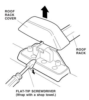
2. Remove the rubber moldings from the front and rear roof rack crossbars. Retain the rubber moldings to be reinstalled later.
