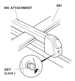
With the ski attached, rock the attachment in all directions to make sure it is installed securely. Adjust as necessary.
