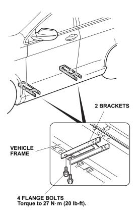
6. Mount the left side step on the left side brackets using four flange bolts and four flange nuts per bracket. Torque the flange bolts to 27 N·m (20 lb-ft).
