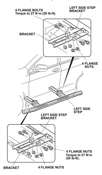
7. Install the left side step brackets to the vehicle frame using two flange bolts per bracket. Torque the flange bolts to 27 N·m (20 lb-ft). On chrome side steps, torque the four flange bolts at the lower part of the left side step to 27 N·m (20 lb-ft).
