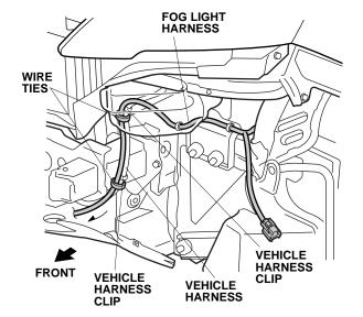
Without a Vehicle Harness: Secure the fog light harness to the vehicle panel using two wire ties with clip.
