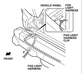
22. Secure the four remaining fog light harness clips to the holes in the vehicle panel.
