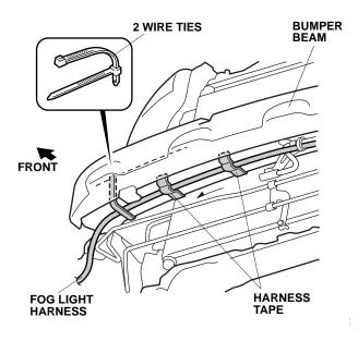
20. Continue routing the fog light harness along the bumper beam to the right side of the vehicle. Secure the fog light harness under the bumper beam using two adhesive tapes and two wire ties connected together. 21. Attach the clip on the fog light harness to the vehicle panel.
