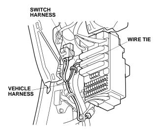
38. Secure the switch harness to the vehicle harness using one wire tie.
