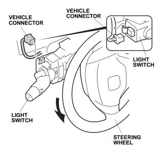
40. Remove the two self-tapping screws from the light switch. While pushing the retaining tab, slide the light switch, and remove it from the steering column. While removing, do not hold the light switch by the lever.
