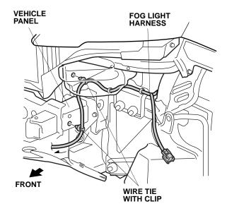
18. Route the fog light harness under the bumper beam towards the right side of the vehicle. Secure the fog light harness.
