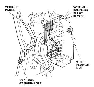
34. Plug the switch harness 2-pin connector into the vehicle harness 2-pin connector. Secure the switch harness to the vehicle harness using two wire ties.
