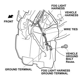
14. Secure the fog light harness to the vehicle harness using two wire ties.
