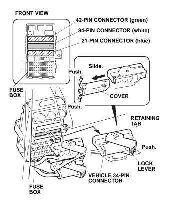
36. Get the fog light switch harness, and insert the white and pink switch harness terminals into the appropriate cavities of the vehicle's white 34-pin connector.
