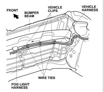
Without a Vehicle Harness: Secure the fog light harness to the bumper beam using two wire ties with clip and one wire tie.
