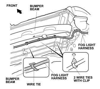
Using isopropyl alcohol on a shop towel, clean the bumper beam surface where the harness tape will attach.
