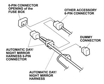
16. Attach a piece of steel wire to the automatic day/ night mirror harness, and route it through the left front pillar trim opening.
