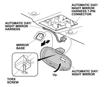
21. Install the day/night mirror on the mirror base, then tighten the T-20 TORX screw installed in the day/night mirror.
