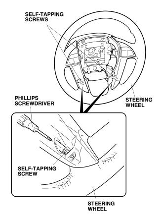
10. Remove the self-tapping screw that fastens the left steering wheel trim and the right steering wheel trim from the steering wheel, and unplug the switch connectors.
