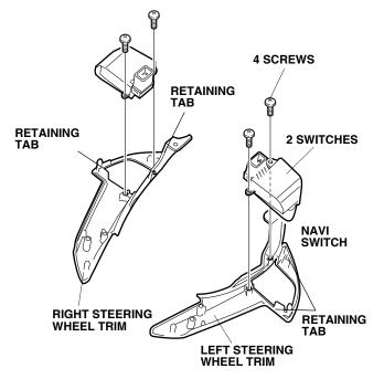
13. Install the two switches to the new left steering wheel trim and new right steering wheel trim with the four screws (reuse). Make sure the retaining tabs are engaged. Go to step 16.
