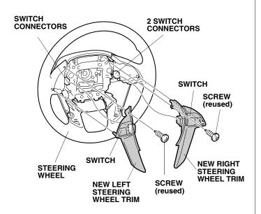
17. Reinstall the two self-tapping screws to the steering wheel.
