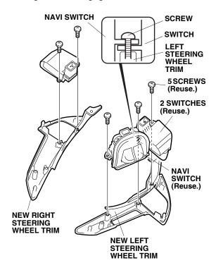
16. Connect each switch connector and install each new steering wheel trim to the steering wheel with the two screws you removed.
