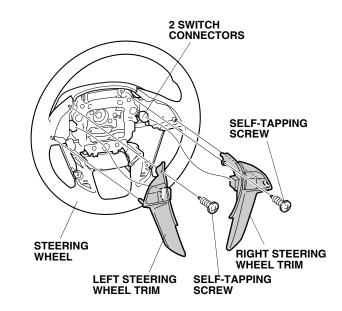
11. Remove the left steering wheel trim and right steering wheel trim from the steering wheel.
