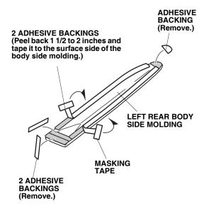
10. Align the end of the left rear body side molding with the rear template as shown and temporarily attach it along the top end of the rear template.
