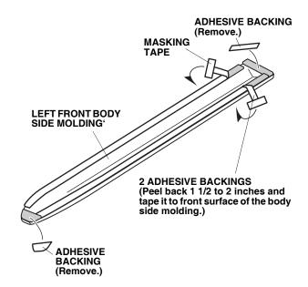
5. Align the end of the left front body side molding with the front template as shown and temporarily attach it along the top end of the front template.
