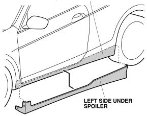
2. Position template A on the vehicle body. Using a felttip pen, mark the vehicle body at the distance shown.
