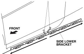
14. Attach the side lower bracket to the vehicle body by pressing it firmly where the double-sided adhesive tape is attached with the palms of your hands or fingers.
