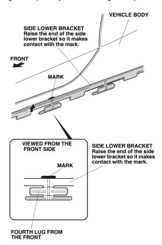
13. Make sure the side lower bracket makes contact with the mark. Apply pressure to the side lower bracket starting from the center and moving to the ends while removing the adhesive backing that was temporarily attached to the lower bracket.
