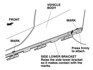
10. Press the front end of the side lower bracket (where you removed the adhesive backing) to attach the part firmly to the vehicle body.
