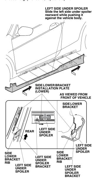
21. Gently tap on the left side under spoiler to remove any gap between the wheel arch of the left side under spoiler and the left front inner fender.
