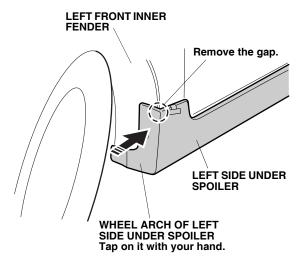
22. Loosely install the two 5 x 18 mm self-tapping screws in the holes in the wheel arch of the left side under spoiler.
