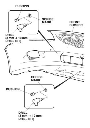
Align the template A with the front bumper as shown. Using a push pin, mark the front bumper as shown. Remove the template A.
