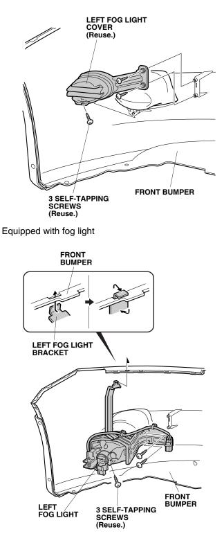
32. Using two self-tapping screws (reuse), eight clips (reuse), four 5 x 18 mm self-tapping screws, and two clips, install the front bumper. Reconnect the fog light harness connectors.
