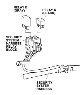
20. Along the door opening, secure the security system harness to the vehicle harness with two wire ties.
