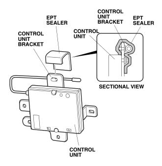
12. Install the control unit bracket onto the bottom of the driver's seat cushion (three self-tapping screws).
