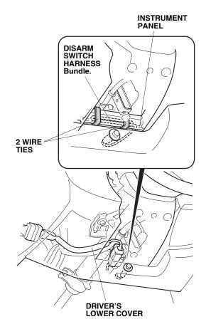
29. Secure the security system harness to the vehicle harness with two wire ties as shown.
