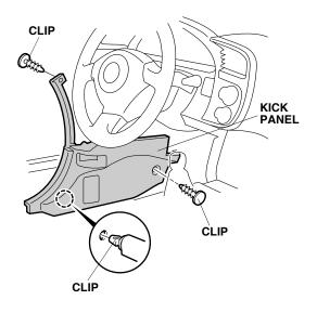
5. Remove the driver's lower cover (turn the knob clockwise, and nine clips).
