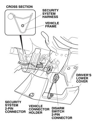
26. Secure the clip on the security system harness to the vehicle frame.
