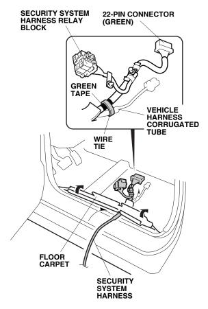
19. Plug relay A (black) and relay B (gray) into the security system harness relay block.
