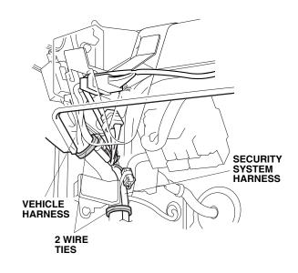
30. Tilt the driver's seat-back forward, then reach under the front of the seat, and plug the 22-pin connector (green) of the security system harness into the control unit.
