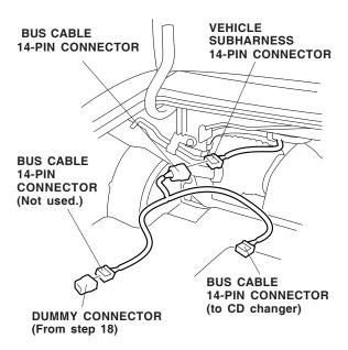
20. Install the dummy connector (from step 18) to the bus cable 14-pin connector.
