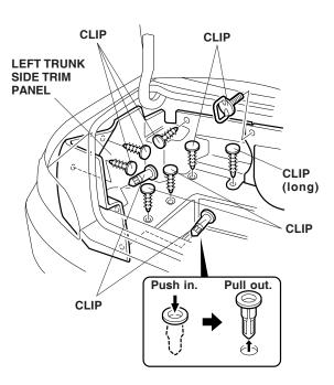
4. Using a tape measure and a felt-tip pen, measure and mark the left trunk side trim panel. Cut out the marked area from the panel with a utility knife.
