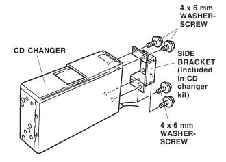
14. Position the CD changer bracket on the CD changer, and secure the bracket with the six 4 x 8 mm washer-screws.
