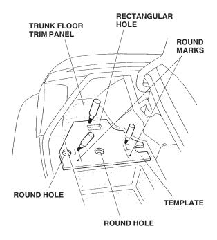
7. While wearing eye protection, lift up the trunk floor trim panel, and drill a 25 mm hole through each of the two marks you made in the panel. Drill the 25 mm holes only through the trunk floor trim panel and not through the trunk floor panel.
