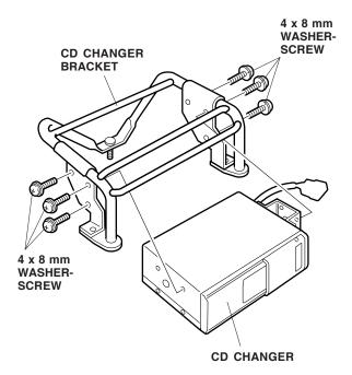
15. Position the CD changer and bracket assembly on the trunk floor panel, and install the two flange bolts from the inside. Install a butyl washer, a plain washer, and a nut on the end of the one stud bolt from the underside, as shown.
