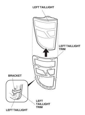
6. While holding light pressure on the trim, carefully remove all of the adhesive backing. After removing the adhesive backing, hold the trim firmly against the taillight with the palm of your hand for 30 seconds.
