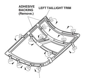
13 ADHESIVE BACKINGS (Peel back 1 1/2 to 2 in. [3-5 cm] of the adhesive backing strips and attach them to the front of the trimwith masking tape.)
