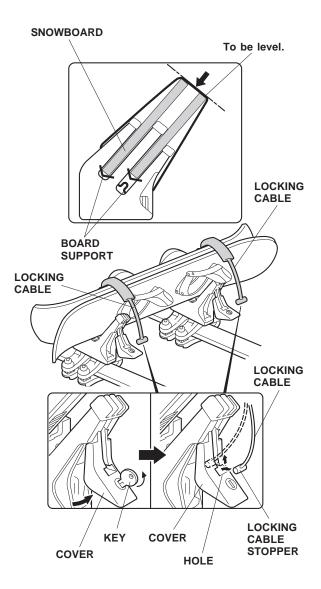
Check that the plate is inserted in the slit securely. Check that the locking cable is inserted in the groove securely.
