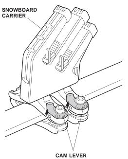
CAM LEVER Return to the original locations. 10. To prevent theft, install the screws in the holes in the top clamps.
