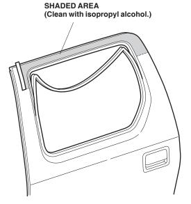
Attach a strip of the masking tape to the ends of the long adhesive backings, and remove 2 to 3 in. (5 to 8 cm) of adhesive backings. Fold back the ends, and tape the ends to the front of the door visor. Remove the short adhesive backing.
