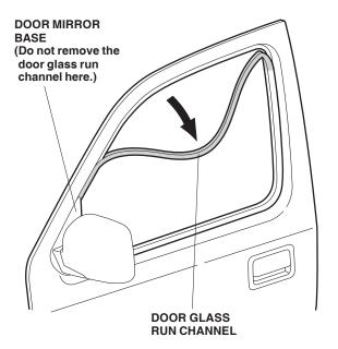
2. Using isopropyl alcohol on a shop towel, clean the shaded area of the door sash.
