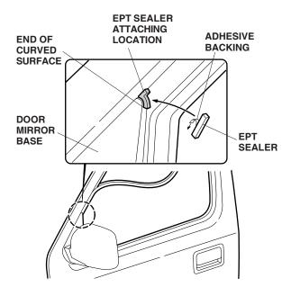
4. Remove the adhesive backing from the EPT sealer and attach it to the door mirror base as shown. The EPT sealer should cover the corner where the mirror and door sash come together. Before you remove the adhesive backing, fit the visor and check that the area where the EPT is positioned completely seals to prevent wind noise. If necessary, adjust the position of the EPT to seal between the door, the mirror, and the door sash.
