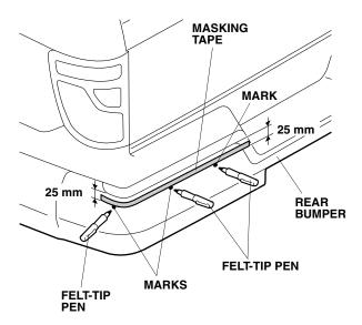
Align and attach masking tape to the marks made on the rear bumper. 12. Attach masking tape at the intersecting point of the seam on the rear bumper and the masking tape attached in step 11.
