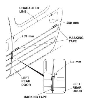
12. On the inside of the left rear upper molding, attach a strip of masking tape to the ends of the long adhesive backing and peel back 1-1/2 to 2 in. (3-5 cm) from the adhesive backing. Tape the ends to the front of the moldings. Remove and discard all other adhesive backings.
