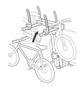
3. Tighten the bicycle arm straps securely around the bicycle frame.
