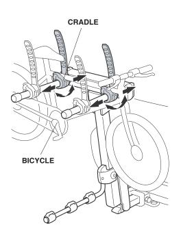
2. When loading two bicycles, alternate the direction of the bicycles.
