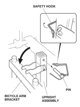
2. Reinstall the pin and safety hook.
