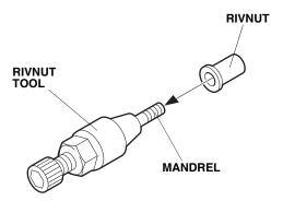
• Insert the rivnut into the hole in the rear under bumper and install the hex wrench on the rivnut tool.
