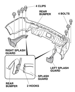
3. Remove the rear lower bumper (four self-tapping screws and twelve hooks).
