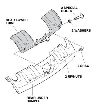
12. Secure the rear lower trim to the rear under bumper with four bolts and two clips.
