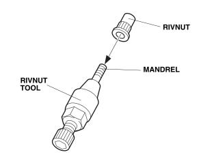
• Insert the rivnut into the hole in the vehicle frame and install the hex wrench on the rivnut tool.
