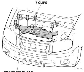
FRONT BULKHEAD COVER 5. Turn the two clips and remove the engine cover as shown.
