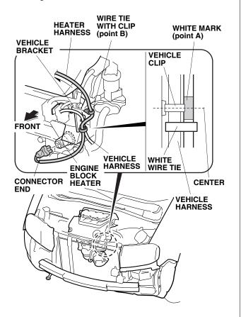
Route the heater harness as shown, and secure it to the vehicle harness with one white wire tie (point A). Secure the one wire tie with clip (point B) to the vehicle bracket. 13. Route the heater harness as shown, and secure it to the fan shroud rib with one black wire tie (point C).
