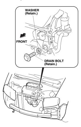
10. Install the engine block heater with aluminum washer into the engine block using a 24 mm socket and a torque wrench. Torque the engine block heater to 60 N·m (6.1 kgf·m, 44 lbf·ft).
