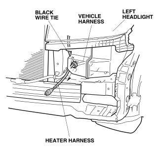
Route the heater harness as shown, and secure it to the vehicle harness with one black wire tie (point F).
