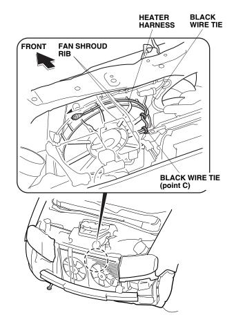
14. Secure the heater harness to the fan shroud rib with one black wire tie.
